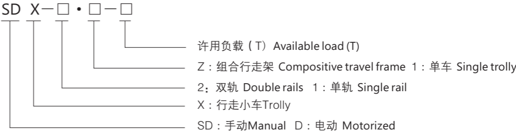
手动双轨组合行走架主要技术参数 Main Tech Data of Manual Dual-rail Combined Travel Frame
